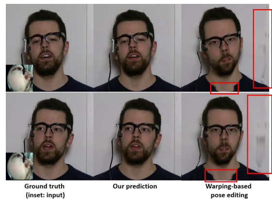
Fig. 22. Comparing our predictions against warping-based head pose synthesis. Here, the target head pose is estimated using [Ruiz et al. 2018] and X2Face [Wiles et al. 2018] drives a single source image by editing its pose. Such an approach generates significant artefacts in the head geometry, as well as in the background and body torso (see red regions).
