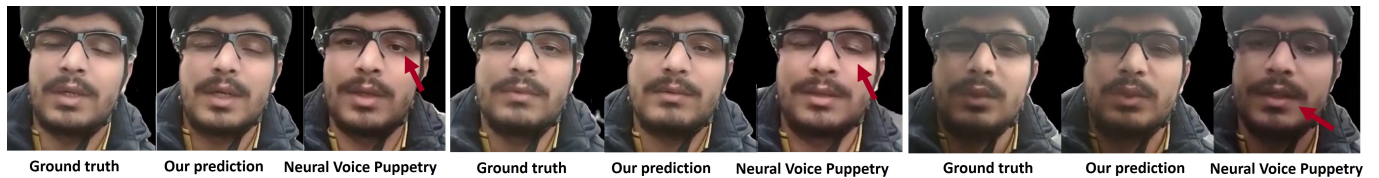
Fig. 19. Neural voice puppetry [Thies et al. 2020] is an audio-driven reenactment solution and hence does not capture ground truth non-verbal expressions (see eye blinks in the first two columns, red arrows) nor scene illumination. It is also sensitive to background audio noise which could lead to inaccurate mouth movements (third column, red arrow). Our approach resembles ground truth more accurately.
