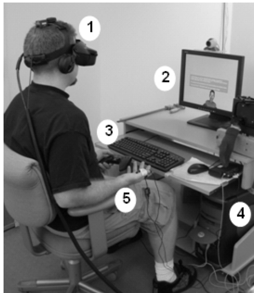
Figure 1. Participant in VR learning environment: 1) Head-Mounted Display (HMD) and orientation tracker, 2) monitor showing the experimenter what participant is seeing in the HMD, 3) Game-pad used to notify agent/avatar, 4) rendering computer, 5) equipment recording skin conductance level (SCL).
